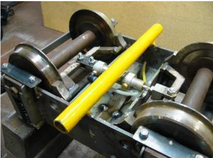
This photo depicts the simplicity to fit a standardised system into a bogie with-out the use of a return spring with operation horizontal and set for axle centre-line block contact at about 80% gross load. The derailment protection / re-rail tube is set to give clearance at solid springs plus an allowance for 3mm tread re-profile (flange profile restoration)
