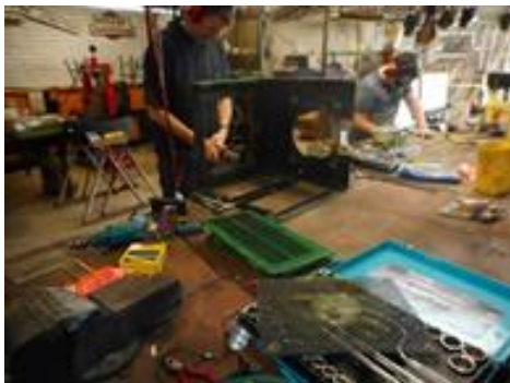
Luke and Xander Prindiville taking the frame apart using a socket set and a Grinder
