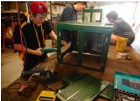
Shaun Elliott drilling the rivets out using a 3mm drill bit so we can use the frames doors again
