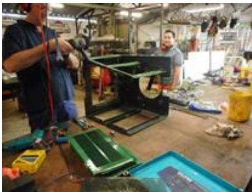
Luke and Xander Prindiville taking the frame apart using a socket set and a Grinder
