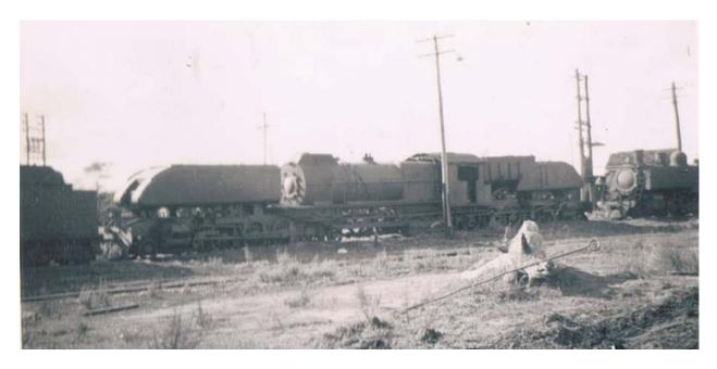
In the above photo the Asg has the hind unit devoid of its return crank rod. There is a "bob" tailed P in front and a Dd behind waiting to enter the Workshops.
