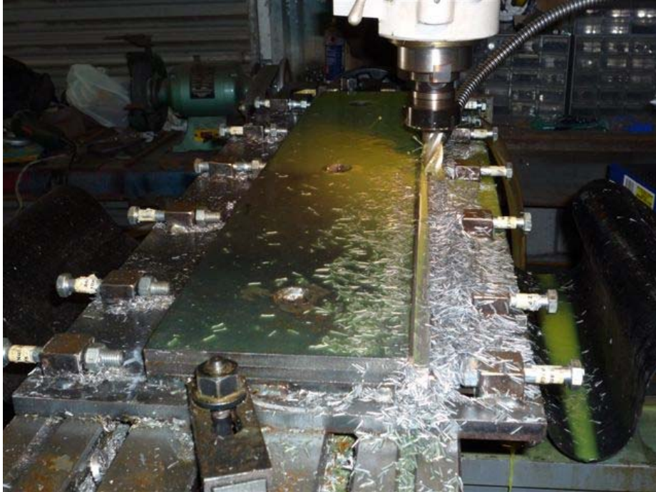
New point blades - the CMR point blade milling jig in action (Photographer: R Stuart)
