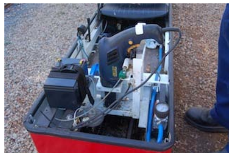
Ingenuity - this loco was powered by a drill
